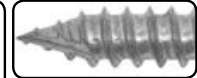
The Type 17 point will clean the existing hole of metal burrs & the oversized threads will generate increased holding strength.
