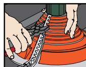
3. Squeeze jointer tightly with pliers to crimp
