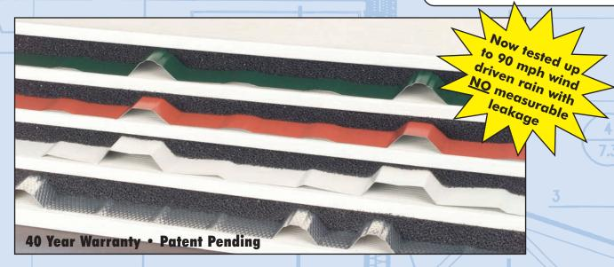
Ultra-Vent will conform to virtually any roof panel configuration. It compresses and fills every void between your ridge cap and the roof panel. Factory applied glue strips allow the installer to roll out Ultra-Vent and apply it to the roof panel, even in windy conditions. Then, any standard ridge cap can finish off the installation.
