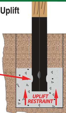
Green Post™ wrap protects in-ground wood applications from the elements. Field tested, the lighter and easier to install Green Post™ double layer wrap is a factory applied heat seal to the lumber, delivered ready to install with uplift restraint system\*. This technique, when used with concrete provides
