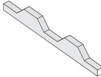
Shaped foam polyethylene (PE) sealing strip.
