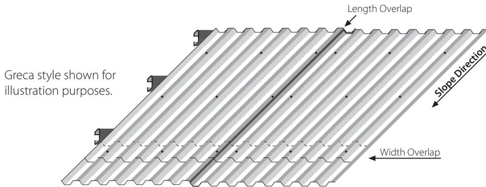
Ceiling installation & fasteners positions
