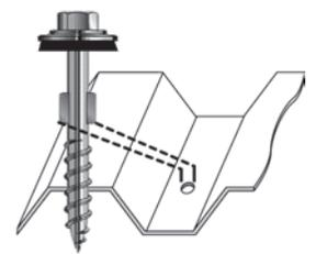
One-Step Fastener eliminates pre-drilling. Creates oversized hole to accommodate expansion and contraction.
