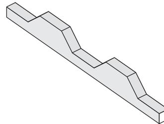
Shaped foam polyethylene (PE) sealing strip.
